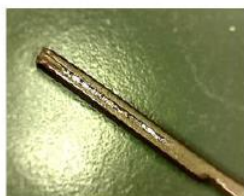
rectum 2 Point corrosion of blade holder
