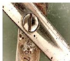
rectum 2 point corrosion of clamp
