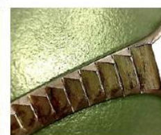
Rectum 2 unlubricated locks - corrosion
