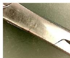
rectum 2 cracked lock, clamp from China
