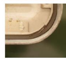
Rectum 2 destroyed lid seal of a container
